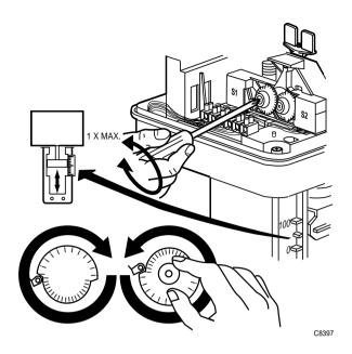
Fig. 6. Adjusting switching points.
